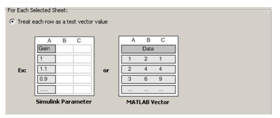
In the first case shown here, column A contains values for the parameter Gain. Suppose this column contains 10 values, in rows 2 through 11 (row 1 is a header). The resulting test vector would be a 1-by-10 array containing 10 values. The first value is 1, the second value is 1.1, etc. The ten populated rows result in a total of ten values, each row being one scalar value.
