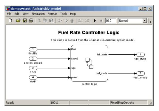
12 In this case, you want to map signals you created in the Test Case Editor to these four Inports in your model. Use the Override Inport Block Signals with SystemTest Data section of the Simulink element.
